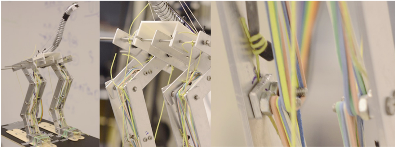
Figure 2. Photograph of the physical model of the skeleton of the guinea fowl. On the left the complete model is shown, on the middle and right sections details of the elastic linkages that are required for the robot to maintain a standing posture can be seen.
