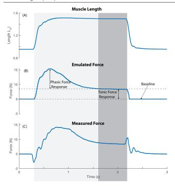
**Figure 5.** Typical force response to ramp-and-hold perturbation with velocity of 300 (degrees  $\rm s^{-1}$ ) is segmented to phasic and tonic intervals. We computed the reflex phasic and tonic amplitudes as illustrated in the figure. The phasic interval was 1400 (ms) long starting at the onset of the perturbation. The tonic interval was 450 (ms) long following the phasic interval: (A) muscle length; (B) muscle emulated force; (C) measured force in the cadaveric tendon.
