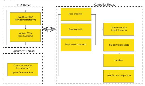
**Figure 4.** Flowchart of the C + + code interfacing the neuromorphic system with the anatomical plant. It is a multithreaded program: FPGA thread read and write signals from and to the sensory and motor FPGAs; the controller thread is a real-time thread for communication to the ADC and DAC cards, implementing the force control PID controller and logging data; the experimental thread is a state machine running the experiments and updating the state of the servo motor perturbing the joint.
