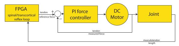
**Figure 3.** The neuro-mechano-morphic design consists of two feedback loops: (i) the spinal and transcortical reflex loops running on FPGA, emulating the stretch reflex mechanism; (ii) the force controller loop, running on C++ to regulate the force output.
