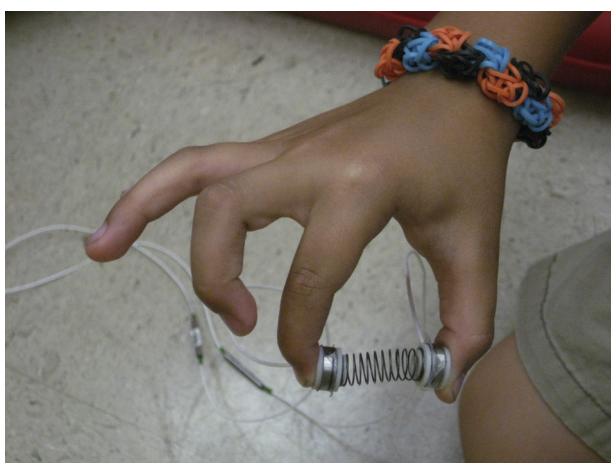
Fig. 2. The S-D test challenges the participant to compress a slender, compliant spring between the thumb and first finger.
