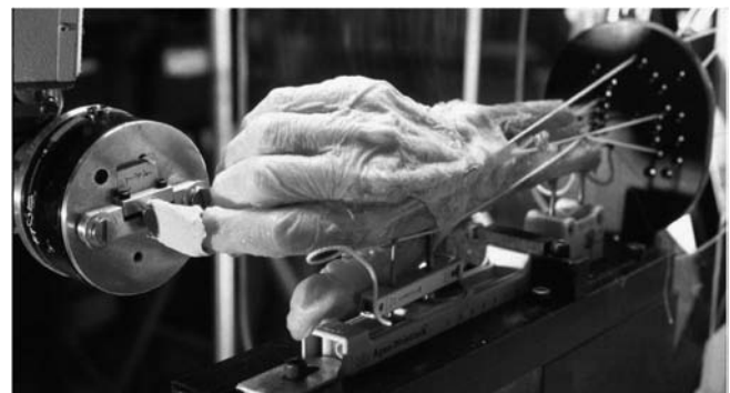
Plate 4 A computer-controlled system to deliver known tensions and displacements to cadaveric hands (Pearlman et al. , 2004; Valero-Cuevas et al. , 2000)
