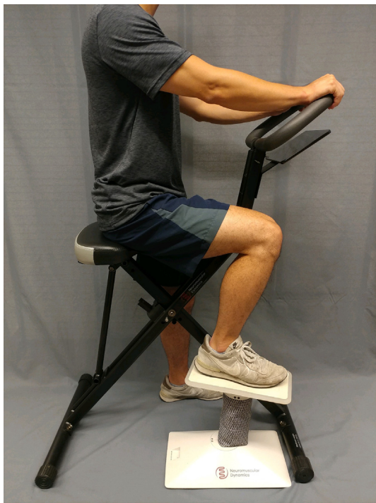
Fig. 1. The lower extremity version of the Valero-Cuevas dexterity test. This test was originally developed for fingers (Dayanidhi, 2013; Dayanidhi and Valero-Cuevas, 2014; Venkadesan et al., 2007), and then adapted into a lower extremity version to quantify the dynamical ability to stabilize unstable foot-ground interactions (Lawrence, 2014; Lyle, 2013).
