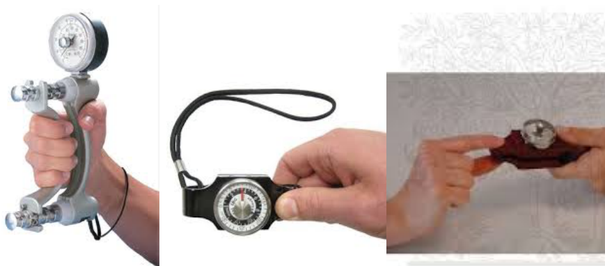
Figure 1.1: Measures of Hand Strength. Grip strength was measured by the dynamometer shown to the left and key (center) and precision (right) pinch strengths were measured as shown with a pinch meter.
