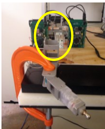
a) Mechanical tendon-driven finger with neuromorphic FPGA controller
