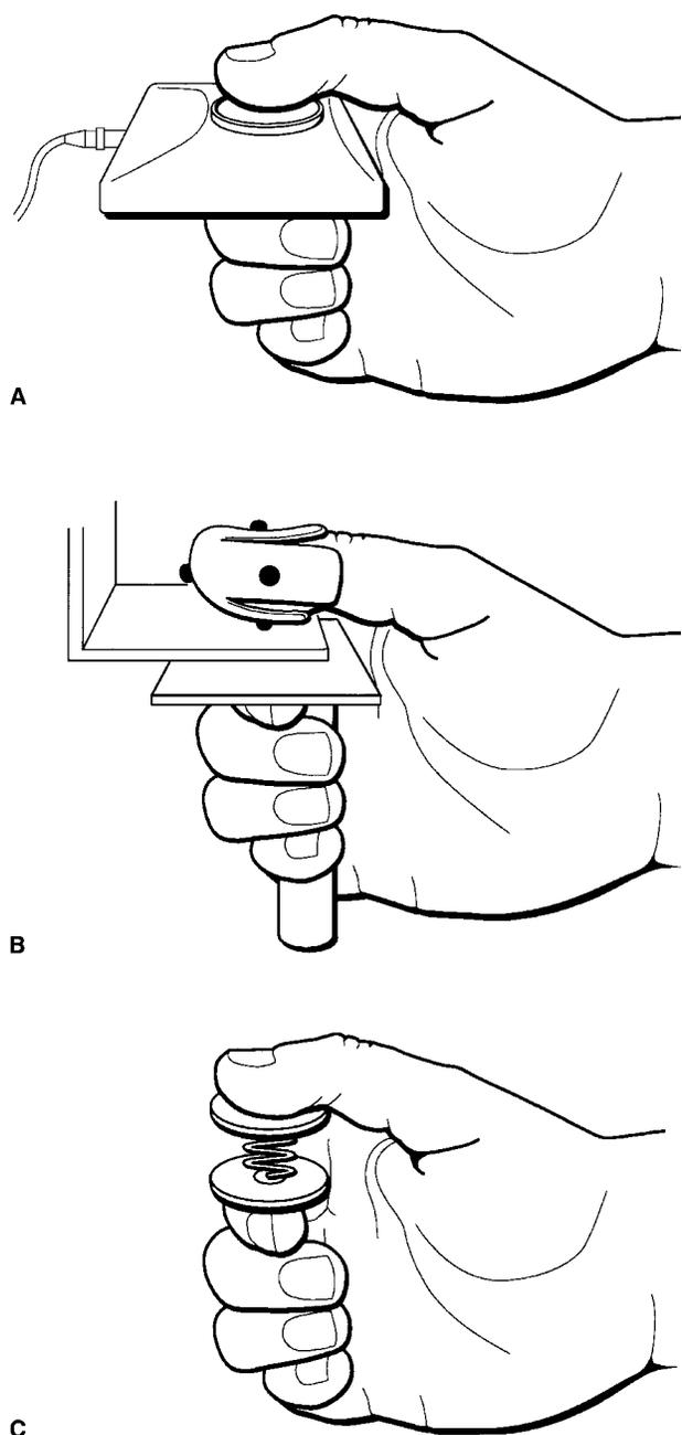
**Figure 1.** (A) Experimental setup for stable tasks using a pinch meter with a concave surface for soft-finger contact to record pinch force. (B) Experimental setup for unstable tasks using a robot-held force sensor and beaded thimble for point-contact to record pinch force. (C) Spring device combining strength and dexterity requirements for dynamic regulation of pinch force.
