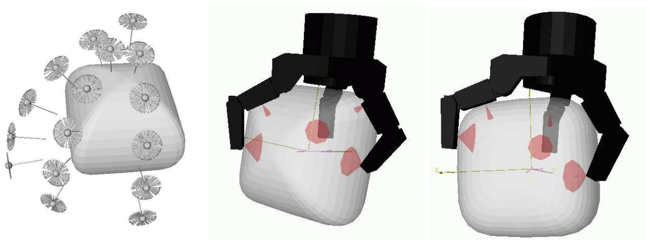
Figure 6: Left: For each superquadric in the training set we generate 1,600 grasp starting poses. These cover 16 positions over 1/8 th of the total surface area, with 100 random combinations of different thumb orientations and finger spread angles. Here the long vector from each point denotes the grasp approach direction and the collection of short vectors shows the various thumb orientations. The spread angle is not shown. Middle: The optimal grasp of the SVM regression function for a superquadric shape previously seen in the training set ( \epsilon_1 = 1, \epsilon_2 = 0.3 ). The quality of this grasp as tested in GraspIt! is 0.402. Right: The optimal grasp of the SVM regression function for novel a superquadric ( \epsilon_1 = 0.6, \epsilon_2 = 0.5 ). The quality of this grasp as tested in GraspIt! is 0.315.
