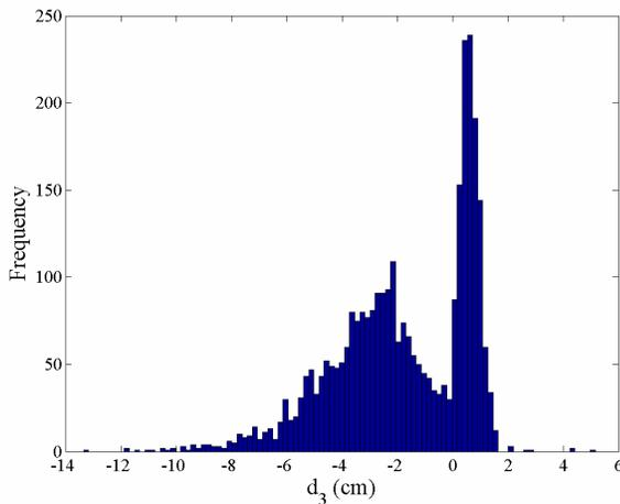
Fig. 1. Histogram of DH parameter  $d_3$ . This is one example of a bimodal distribution that resulted from the MC simulations. The distribution was characterized as a mixture of normal distributions, specified in the  $d_3$  cell of Table 1.
