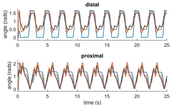
Fig. 4. The desired (black), open-loop (blue), and close-loop (orange) joint angles for one trial of the cyclical movements in-air task.
