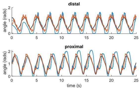
Fig. 8. The desired (black), open-loop (blue), and the close-loop (orange) joint angles for one sample run of the locomotion with the gantry task.
