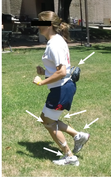
Figure 2.6: Subject wearing five accelerometers attached to the thighs, trunk and ankles.
