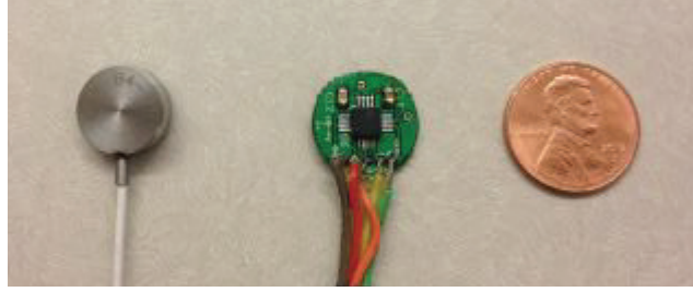
Figure 2.2: Uni-directional load cell and tri-axial accelerometer next to a US penny for size comparison.
