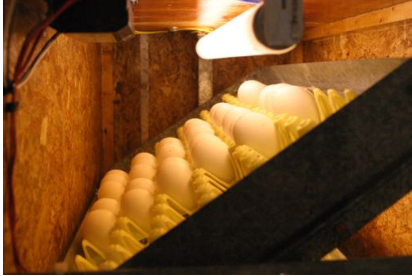
Figure 6.1: The incubator. Note that the surface holding the eggs was rotated at 2-hour intervals to ensure equal light exposure.
